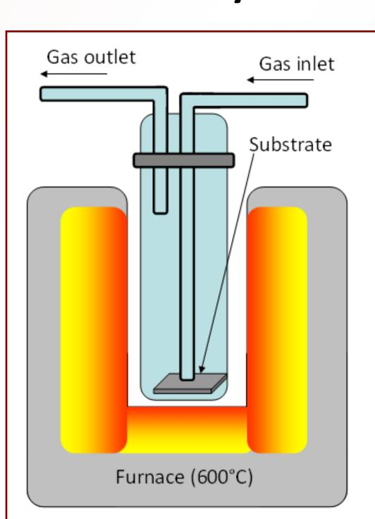
The heat dissociates the molecule and lead to element atom layer by layer deposition on the surface.
